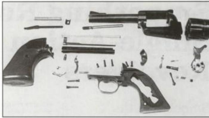
The three-screw action and firing mechanism components, fully disassembled. The three-screw actions are easier to work and produce better actions for the effort than do the two-screw mechanisms.
