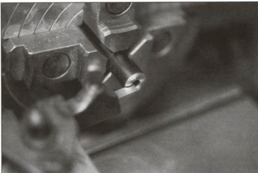
Setup for a barrel in the adjustable-jaw chuck. The ¼-inch radius tool will form a standard factory crown. With a different tool bit and the tool post turned, a recessed or target-style crown can be applied.
