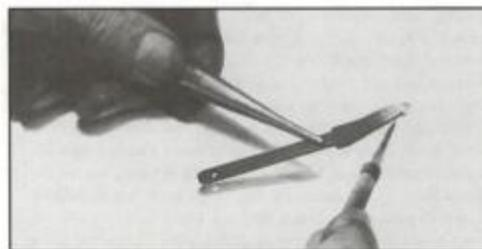
Above right: The head of the hammer strut should be polished. You should also deburr and polish the shank of the hammer strut that runs through the hammer spring and seat/retainer.
