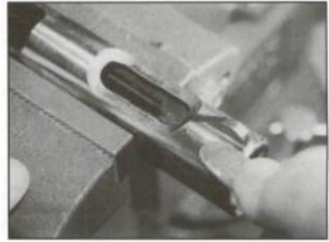
A soft stone is used when cleaning up after silver soldering on a custom front sight, so that it will contour into the square joint. Using a crisscross motion keeps you from wearing in flat spots on round surfaces.
