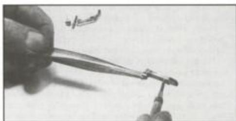
Above left: Polish the rear of the hand and the front below the lower tooth. Don't change the dimensions of the top.
