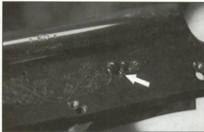
If carrier screws are switched during reassembly, the lock screws won't line up properly.
