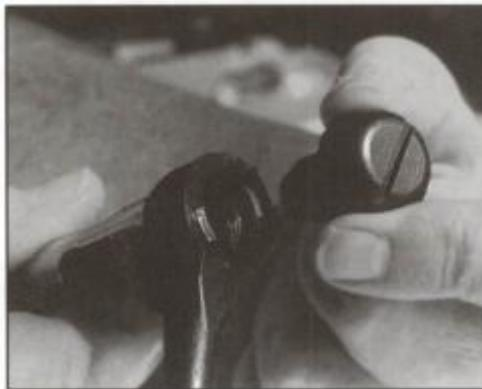
Removing the bolt-assembly screw allows you to get at all the insides for additional cleaning.
