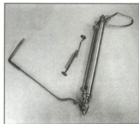
This improvised spring-rate jig can be used with your trigger scale. It's more precise than using a postal scale.
