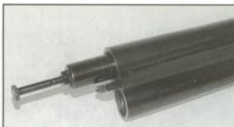
As this simple chamber gauge shows, the chamber on this double gun is short by today's standards. If a 2 $\frac{3}{4}$ -inch shell is fired in this chamber, the shell will open into the forcing cone causing extremely high pressure and damage to the shot column. The result will be excessive recoil and poor patterns.
