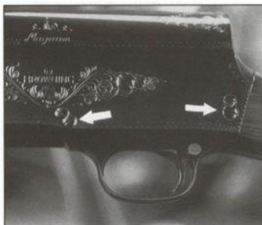
Drifting out the trigger assembly and lock screws allows removal of the entire trigger group. It usually isn't necessary to completely disassemble this group.
