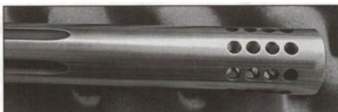
Some Volquartsen heavy stainless steel barrels come with integral muzzle compensators, which have eight rows of four  $\frac{17}{64}$ -inch diameter holes to vent powder gases.
