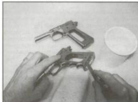
When stoning the inside of a flared magazine well with a coarse, soft stone, move the stone linearly and axially and use water liberally to remove fouling. Using a coarse stone, of course, removes more metal, but it also reduces your stoning time.
