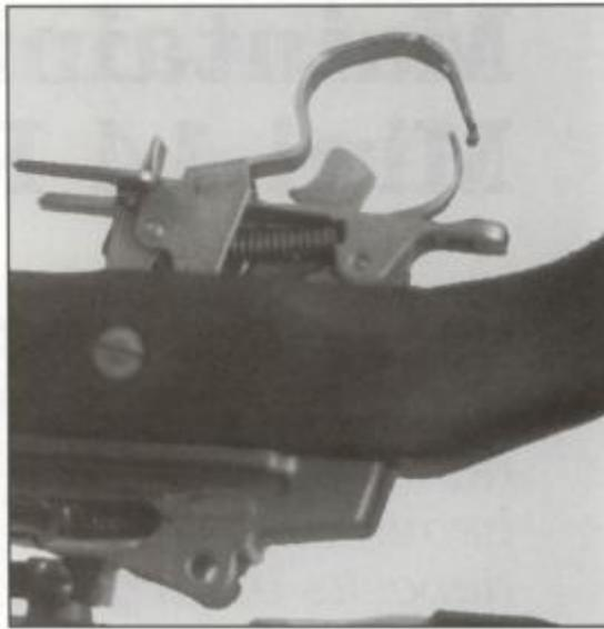
Pulling up on the rear of the trigger guard and pivoting it forward will allow the removal of the trigger group.
