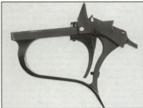
Left — This shows the striker being retained by the trigger notch. The two parts' engagement is seen to the right of the tallest portion of the trigger group. That tall feature guides the trigger group into the receiver. The trigger overtravel and freeplay screws are seen to the lower right and in the middle pointing forward and up, respectively. The trigger return spring cup is above the freeplay adjustment screw.
