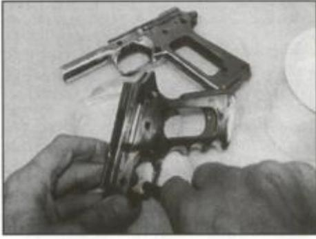
Stoning the inside of a trigger guard and the finger grooves on the frontstrap with a rocking boat motion are good ways to use a soft stone. Strokes along a curved surface tend to cause less trouble than trying to rock against the curve.
