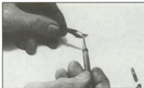
Right — The rear of the trigger beneath the sear area must be polished as well.
