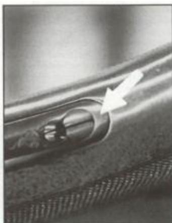
Stock tang screw removal should let the stock come off. If not, a few whacks with a rubber mallet should do the trick.
