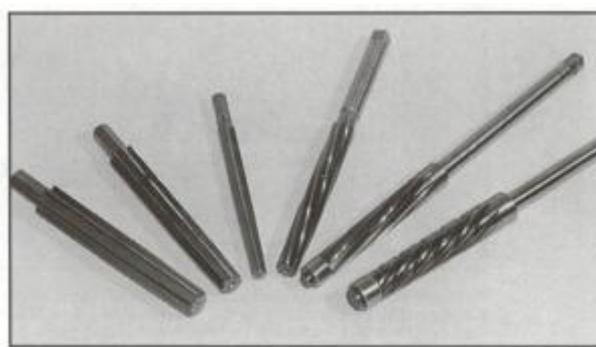
This is an assortment of long forcing-cone chamber reamers. The three on the left are the straight fluted reamers available from Brownells. The next item is a 28-gauge spiral fluted tool made by Clymer Manufacturing. On the right are two spiral fluted solid carbide reamers made by J.G.S. The solid-carbide tools are harder than chrome, and they allow you to lengthen chambers without having to remove chrome after the job is done.
