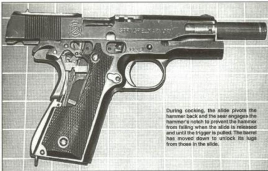
During cocking, the slide pivots the hammer back and the sear engages the hammer's notch to prevent the hammer from falling when the slide is released and until the trigger is pulled. The barrel has moved down to unlock its lugs from those in the slide.
