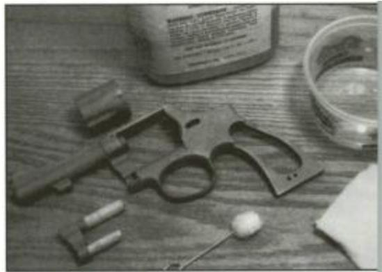
If you bead-blast the gun you're going to blue, be sure to mask off any bearing areas that don't need to be roughened. After blasting, the gun is ready for the cold blueing.
