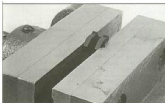
Pushing a file over a flat-topped vise will keep the edges of the part from rounding over.
