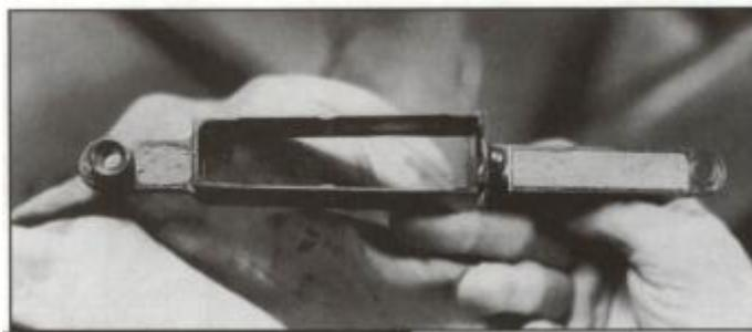
Any areas on the receiver that might get hung up in the glass — like the upper portion of the trigger guard and the magazine assembly — should be packed with children's modeling clay.
