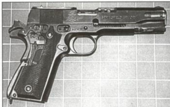
In battery with the hammer and sear engaged and the barrel locked up, the pistol will not fire until the grip safety is depressed and the thumb safety is engaged in its frame notch.
