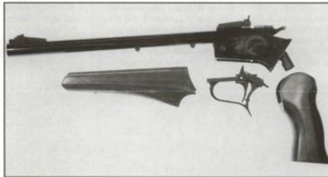
The Contenders unusual geometry allows the complete trigger group to be taken out of the receiver and worked on separately. It's best to work on this trigger group and leave the regular sear and hammer alone, because extremely good results can be achieved without any work being performed on the parts lodged within the receiver.
