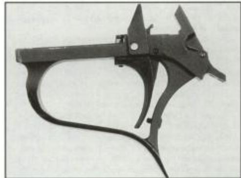
Right — This shows the trigger striker in the released position.
