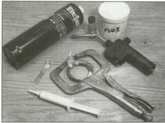
Equipment most used in silversoldering includes propane, flux, torch heads, clamps, silversolder wire, silver ribbon, a silversolder paste syringe, and solder-masking liquid.
