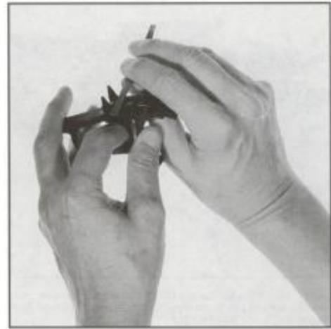
Use a Brownells flexible stone strip to smooth the underside of the trigger notch without disassembling the trigger group. This is done to smooth the trigger's feel without significantly reducing the trigger pull. Be sure to remove all the grit from the action if you perform this work on an assembled trigger group.
