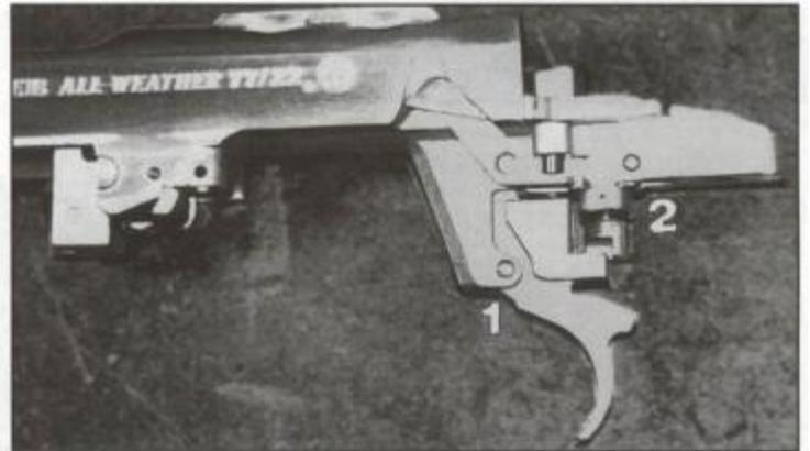
The trigger/sear assembly of a 77/22 is taken down by pushing out two pivot pins — the trigger pivot pin (1) and the sear pivot pin (2) — with a proper size drift punch.
