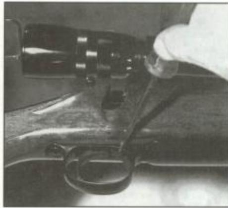
The bolt-stop is located inside the trigger guard, just in front of the trigger as shown by the pointer. The magazine floorplate is opened by pressing on the release button directly to the right of the pointer.
