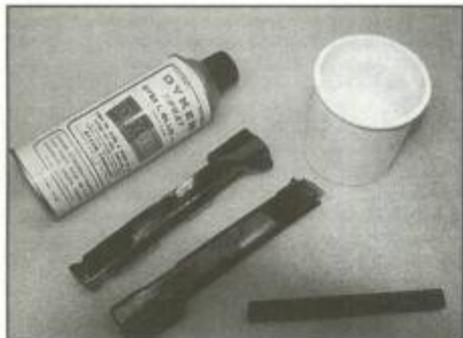
Dykem steel dye is often used to identify high areas when stoning with a flat stone. For the gunsmith on a budget, dark permanent-felt markers serve as well. Use a wide, flat, hard stone such as a medium-hard Carborundum to level flat surfaces.
