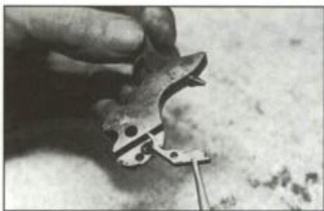
This photo shows the relationship of the hammer to the cylinder-stop as the hammer is being cocked.
