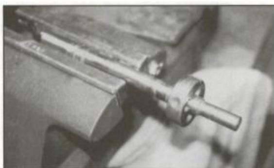
The die for an autopistol is located on the barrel-threading guide just before starting on the barrel. Note the drive indentation on the outside of the die by which the die wrench is to grip and drive the die.
