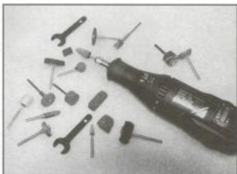
The Dremel Moto-Tool, shown with an assortment of mounted stones, Cratex, cutoff wheel and sanding drum, is a favorite in the author's gunsmith shop. Of course, gunsmiths should always wear eye protection when working with rotary power tools.
