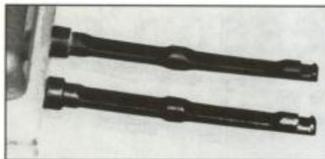
This reworked extractor hook (bottom) had the base of its slot beveled and a notch cut into the slot's lower front. The lower front edge of the hook was slightly relieved. Compare this to the unaltered extractor on the top.
