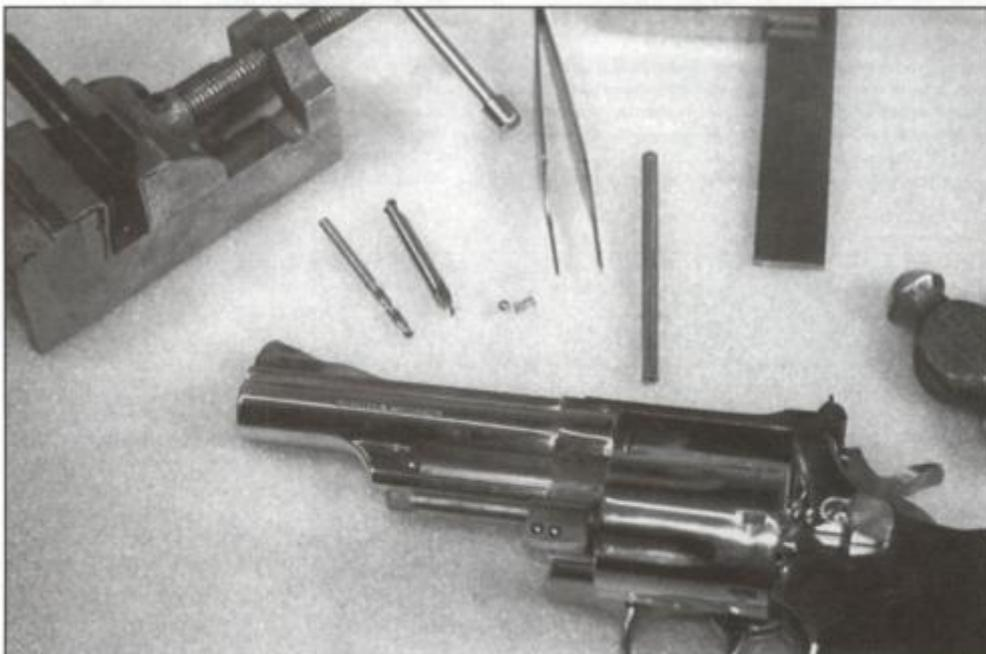
To fix erratic shot placement in revolvers, consider tuning the lockup between the crane and the receiver. This Model 66 S&W pistol has two crane balls installed. The hardest part of the installation was gripping the crane while drilling and staking the top of the hole.
