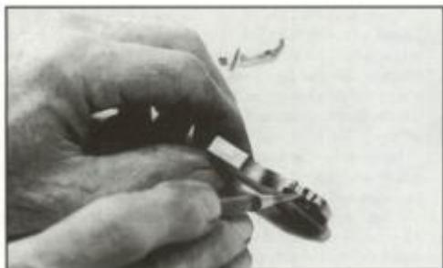
Left — The first place to start is to polish the face of the hammer hooks and hammer toe. This applies to old or new Ruger actions.
