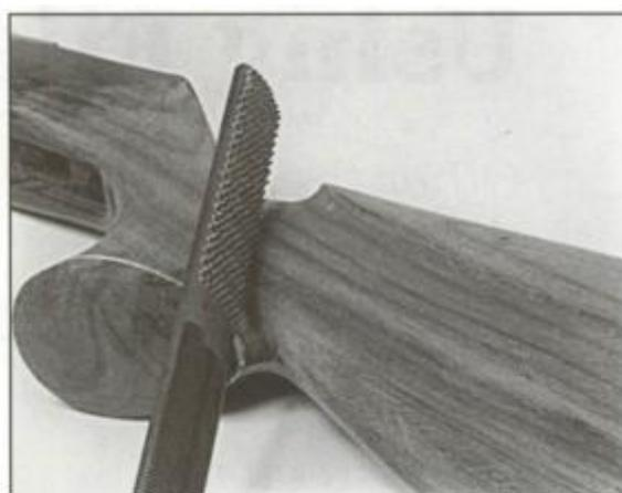
The horseshoe rasp has a curved side and a flat side. It comes in handy when roughing out gunstock shapes.
