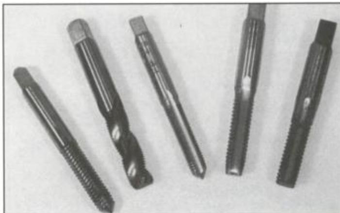
Interrupted roll, spiral-fluted, taper, plug, and bottoming are the main types of taps.
