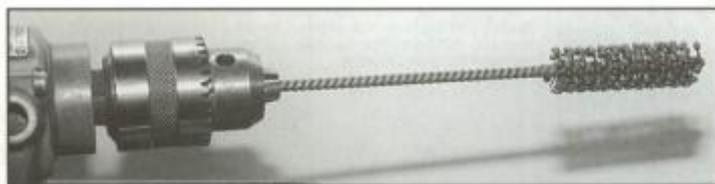
The ball-type brake cylinder hone is a great tool for finishing a long chamber forcing cone. These are readily available at any auto parts store. Be sure to use one that fits tightly in your newly-machined forcing cone.
