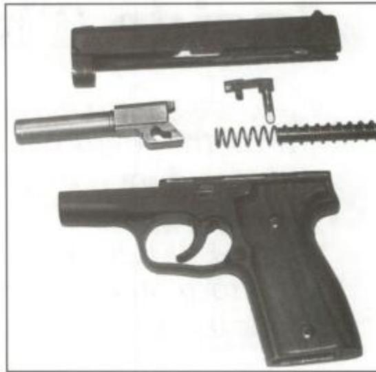
Field stripping is as far as the factory wants anyone to go in disassembling the K9, and Kahr will void the warranty if a gun is damaged or malfunctions due to improper reassembly.
