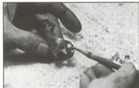
Stoning and polishing the cylinder-stop cam bevel eases the revolver's operation and prevents breakage of the stop legs.
