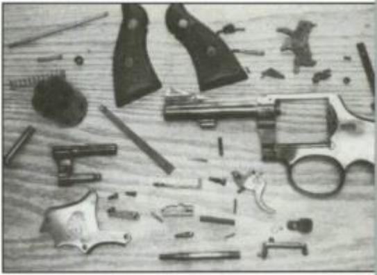
The author used a Smith & Wesson revolver for this project. The gun needs to be fully disassembled before blueing.
