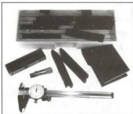
You'll need some specialized tooling designed for frame-to-slide fitting. Top to bottom and left to right are a set of frame rail bars, a magazine well filler, slide micrometer, slide spreaders, frame side plates and dial calipers, all available from Brownells.
