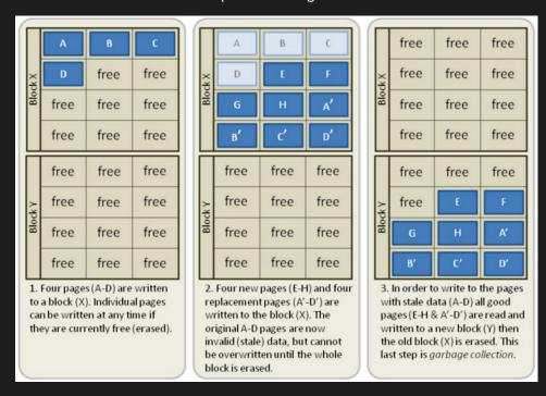
As you can see in the above illustration, data (from a file) will be written to the four first pages of Block X. Later new data will be written to the remaining pages and the data from the first files will be marked as invalid (for instance by a Trim operation when deleting a file). As explained on https://en.wikipedia.org/wiki/Trim\_(computing) [Wikiless] [Archive org]; the erase operation can only be done on entire blocks (and not on single pages).
