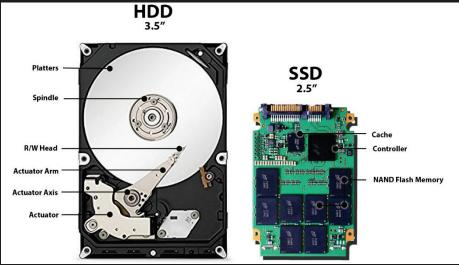
If you intend to wipe your whole HDD laptop, the process is rather straightforward. The data is written at a precise location on a magnetic (hard) platter (why it is called a hard drive) and your OS knows precisely where it is on the platter, where to delete it, and where to overwrite it for secure deletion using simple processes (like just overwriting that location over and over until no traces are left).
