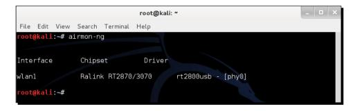
**4.** Now enter airmon-ng start wlan1 command to create a monitor mode interface corresponding to the wlan0 device. This new monitor mode interface will be named mon0. (You can verify if it has been created by running airmon-ng without arguments again).
