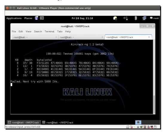
**20.** Once enough data packets have been captured and processed, aircrack-ng should be able to break the key. Once it does, it proudly displays it in the terminal and exits, as shown in the following screenshot:
