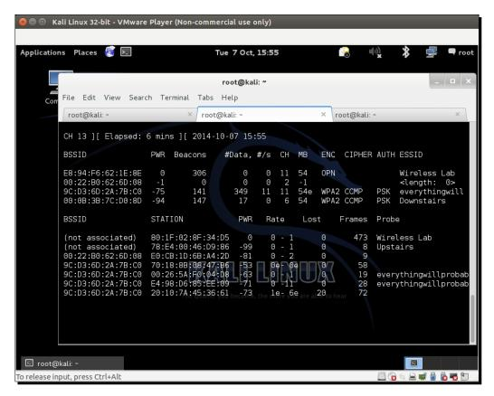
**9.** Even airodump-ng is unable to discern that there are actually two different physical access points on the same channel. This is the most potent form of the evil twin.
