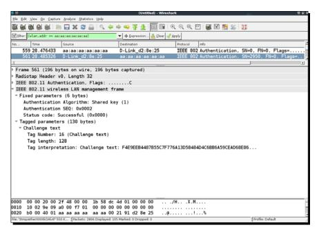
**9.** In the third packet, the tool sends the encrypted challenge to the access point:
