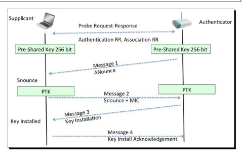
To crack WPA, we need the following four parameters from the four-way handshake— Authenticator Nounce, Supplicant Nounce, Authenticator MAC, and Supplicant MAC. Now, the interesting thing is that we do not need all of the four packets in the handshake to extract this information. We can get this information with four packets; packets 1 and 2 or just packets 2 and 3.
