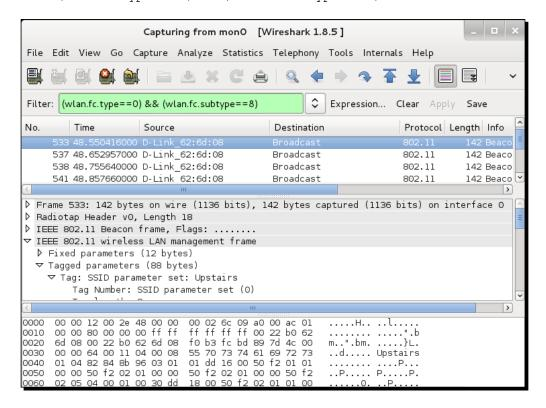
5. Alternately, you can right-click on any of the header fields in the middle window and then select Apply as Filter | Selected to add it as a filter.
