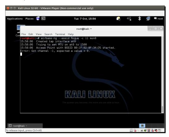
**4.** This new access point also shows up in the airodump-ng screen.. It is important to note that you will need to run airodump-ng in a new window with the following command:
