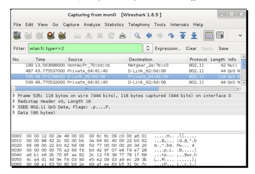
4. To additionally select a sub-type, use the wlan.fc.subtype filter.
