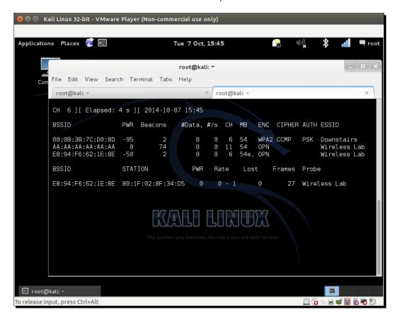
**3.** Using this information, we create a new access point with the same ESSID but a different BSSID and MAC address using the airbase-ng command. Minor errors may occur with newer releases:
