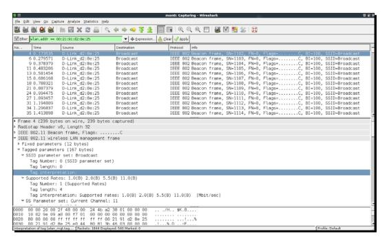
**4.** In order to bypass Beacon frames, we will first use the passive technique of waiting for a legitimate client to connect the access point. This will generate probe request and probe response packets that will contain the SSID of the network, thus revealing its presence:
