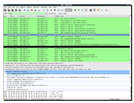
**7.** We can easily locate the HTTP post request that was used to send the password to the wireless access point:
