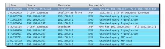
**2.** Apply a Wireshark filter for DNS and, as we can see, the victim is making DNS requests for https://www.google.com:
