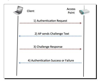
The wireless client sends an authentication request to the access point, which responds back with a challenge. The client now needs to encrypt this challenge with the shared key and send it back to the access point, which decrypts this to check whether it can recover the original challenge text. If it succeeds, the client successfully authenticates; if not, it sends an authentication failed message.
