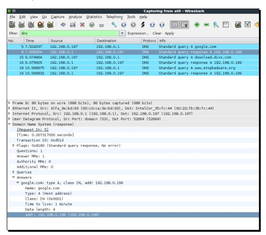
**5.** On the victim's machine, we see an error that says **Unable to connect**. This is because we made the IP address for <code>google.com</code> as <code>192.168.0.199</code>, which is the hacker machine's IP, but there is no service listening on port 80:
