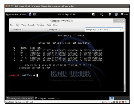
**21.** It is important to note that WEP is totally flawed and any WEP key (no matter how complex) will be cracked by Aircrack-ng. The only requirement is that a large enough number of data packets, encrypted with this key, are made available to aircrack-ng.
