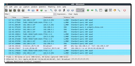
**10.** Let's now ping the gateway 192.168.0.1 from the client machine. We can see the packets in Wireshark (apply a display filter for ICMP), even though the packets are not destined for us. This is the power of man-in-the-middle attacks:
