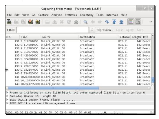
**4.** These are wireless packets that your wireless adapter is sniffing off the air. In order to view any packet, select it in the top window and the entire packet will be displayed in the middle window.
