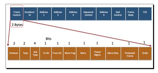
The Type field defines three types of WLAN frame:
