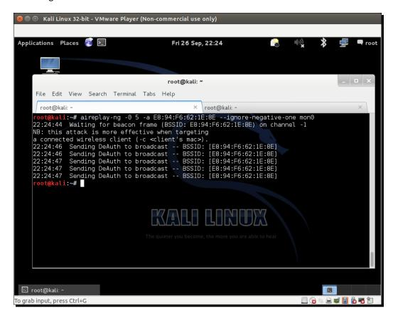
**4.** Note how the client gets disconnected from the access point completely. We can verify this on the airodump-ng screen as well:
