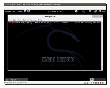
**10.** We will request airodump-ng to save the packets into a pcap file using the --write directive:
