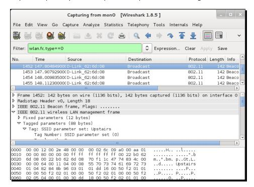
2. To view Control Frames, modify the filter expression to read wlan.fc.type == 1.
