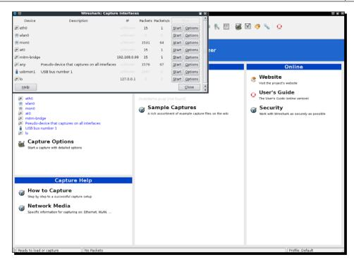
2. Start sniffing on the at0 interface so that we can monitor all traffic sent and received by the wireless client:
