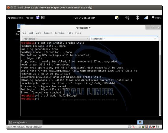
**3.** We will then add both the Ethernet and the At 0 virtual interface created by Airbaseng to this bridge:
