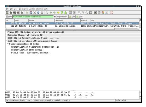
**8.** The second packet consists of the access point sending the client challenge text, as shown in the following screenshot:
