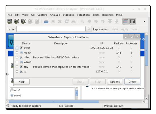
**3.** Select packet capture from the mon0 interface by clicking on the **Start** button to the right of the mon0 interface as shown in the previous screenshot. Wireshark will begin the capture, and now you should see packets within the **Wireshark** window.
