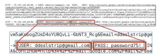
This attack is only effective from the same Layer 2 network segment. However, it is successful on both wired and wireless networks. Although the ARP redirect can be applied against a network segment, such an attack will impact the network bandwidth, which may be detected. Therefore, it is most effective to direct this attack against single devices.
